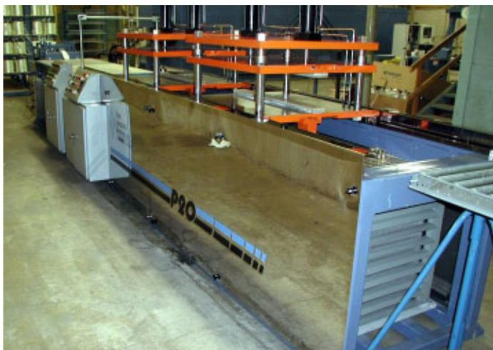
Entec Composite Machines has recently upgraded its line of pultrusion machines to use an electronic motion controller. To replace the old PLC-driven velocity controls, Entec selected a programmable motion controller from Delta Computer Systems to output a variable control voltage to each of the two proportional servo valves of the pulling cylinders in order to precisely
